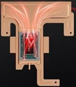
Figure 6: Vapor Chamber and Cooling Mesh - Highlights the advanced cooling features of the SER7.
