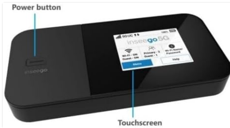
Figure 2.2: Top-down view highlighting the power button and the interactive touchscreen display.
