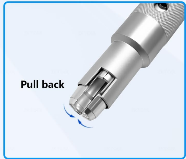
Image 4.1: This diagram illustrates the adjustment mechanism of the puller. The side opening can be adjusted by pushing up to stretch out the jaws and pushing down to pull them back, allowing for a firm grip on the injector.
