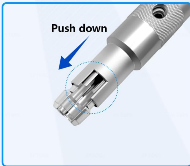
Image 4.1: This diagram illustrates the adjustment mechanism of the puller. The side opening can be adjusted by pushing up to stretch out the jaws and pushing down to pull them back, allowing for a firm grip on the injector.
