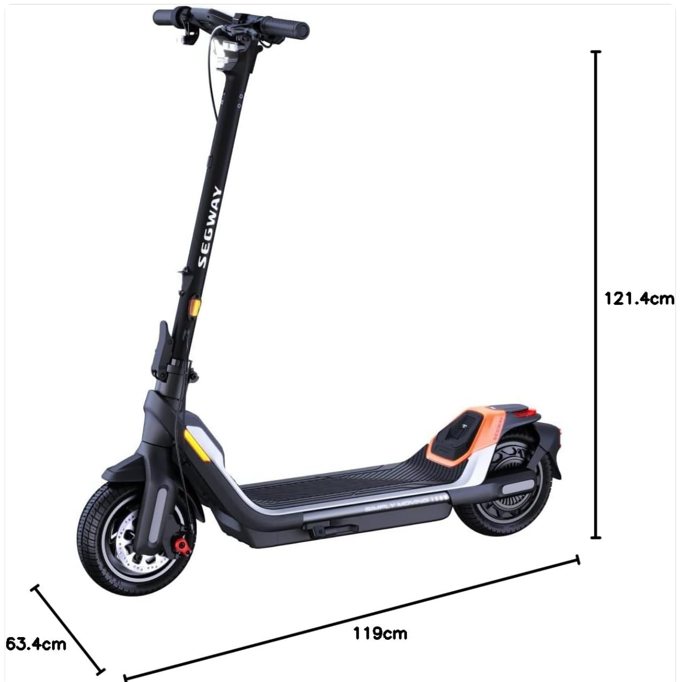
The Segway Ninebot P65A Electric KickScooter displayed with its key dimensions: length (119 cm), width (63.4 cm), and height (121.4 cm).
