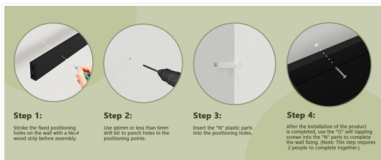
Figure 5.1: Wall mounting steps.
