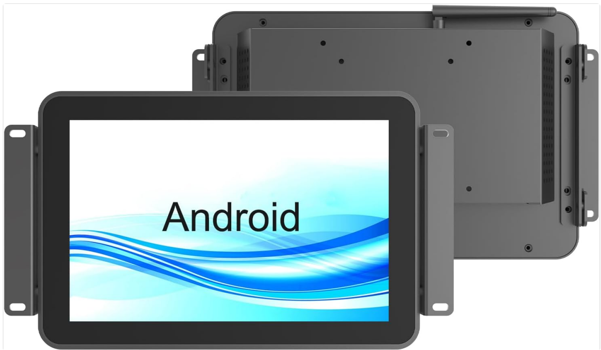
Figure 2.1: Front and rear view of the GreenTouch 10.1-inch Open Frame Android Touchscreen Monitor PC.
