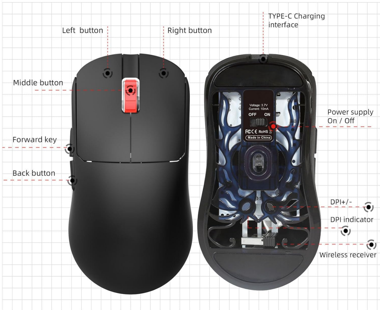
Image: A detailed diagram illustrating the various buttons and components of the mouse, including the left button, right button, middle button (scroll wheel), forward key, back button, Type-C charging interface, power supply switch (On/Off), DPI indicator, DPI+/- buttons, and wireless receiver storage slot.
