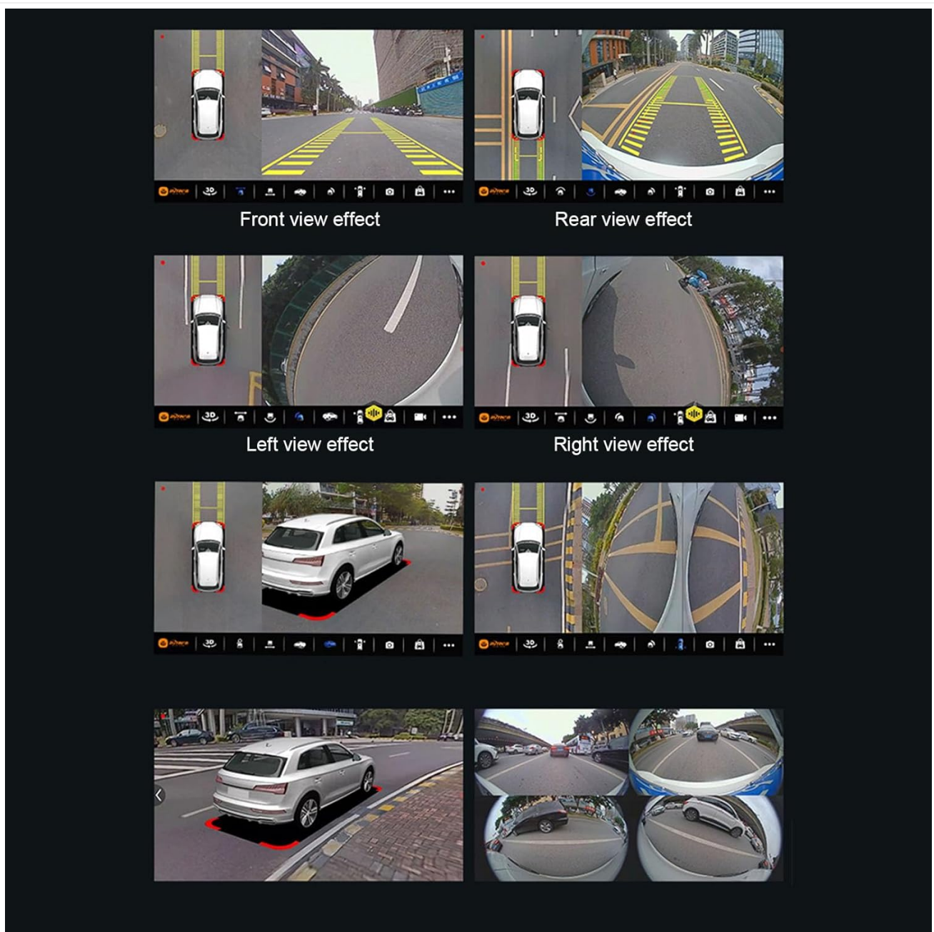
Image 6.1: Examples of the panoramic surround view display, showing front, rear, left, and right camera perspectives, as well as a combined overhead view.
