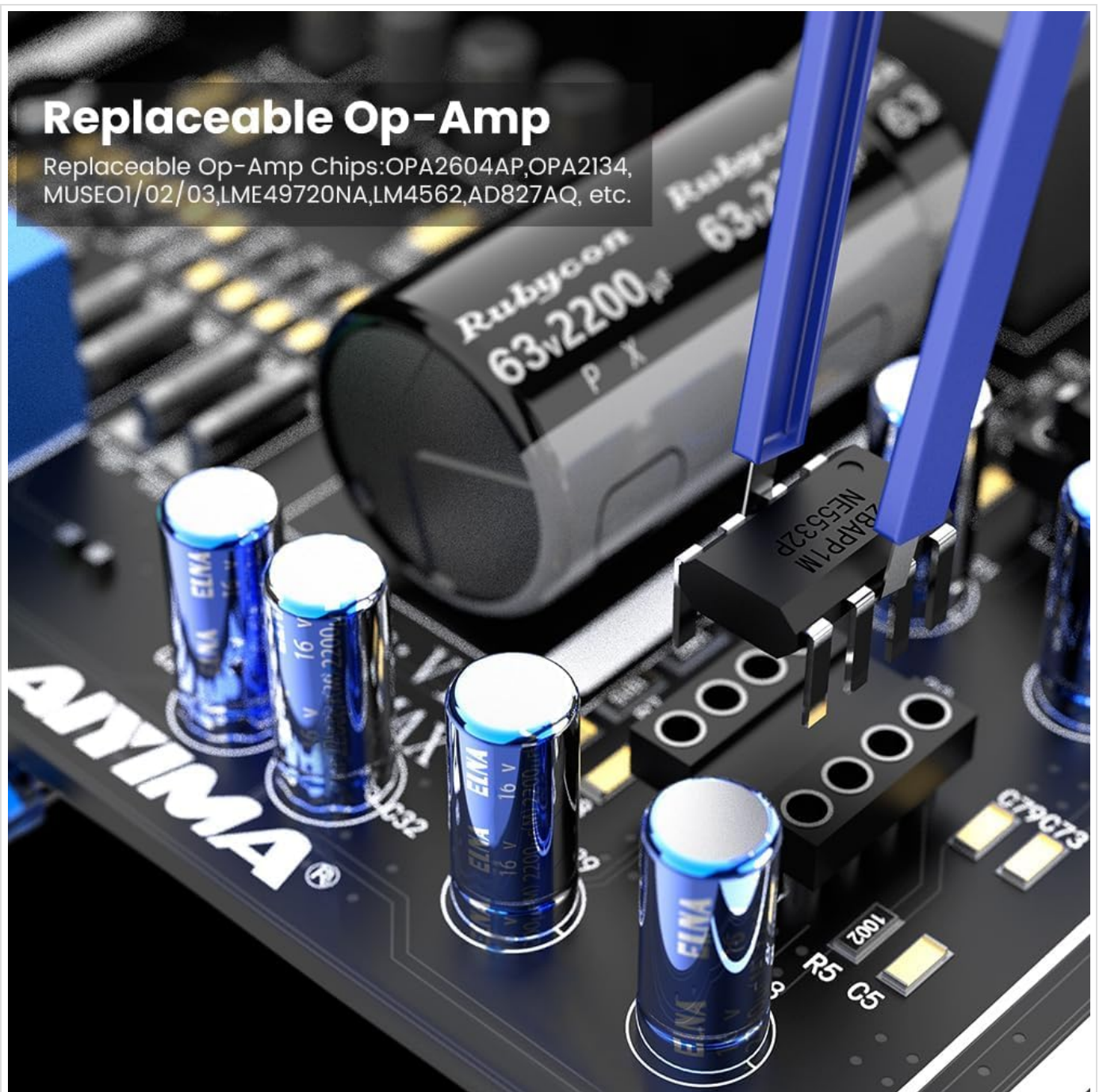
Figure 6: Detail showing the replaceable Op-Amp on the amplifier's circuit board, indicating compatibility with various DIP8 dual op-amps.
