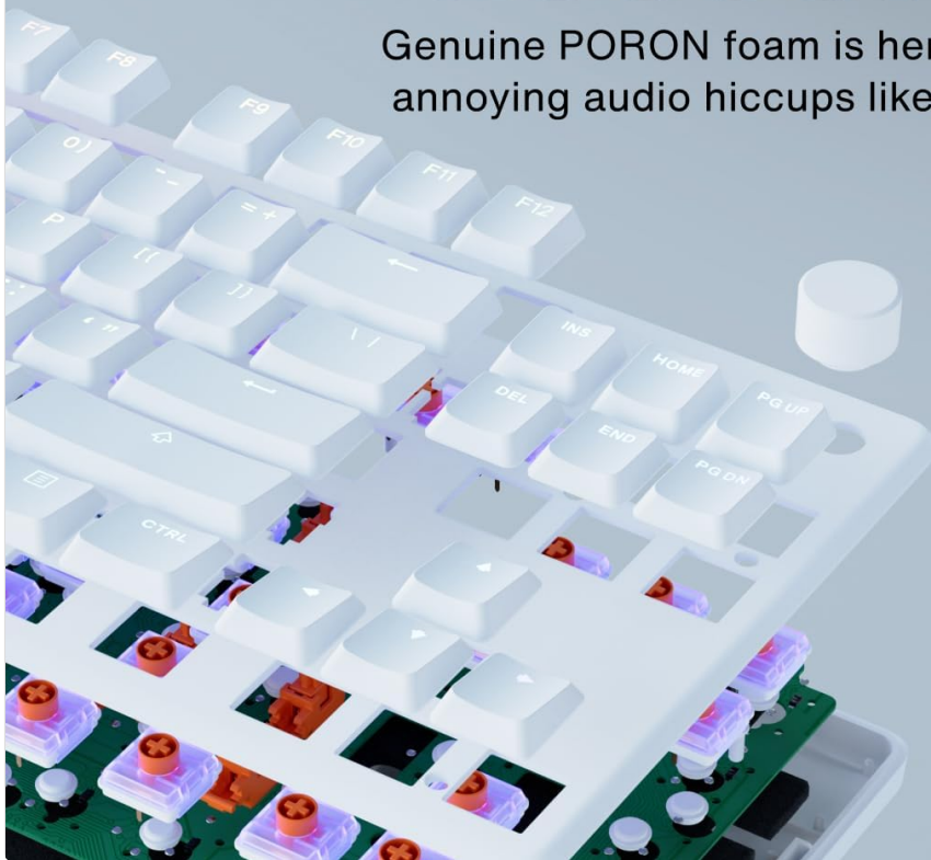
Image 4.5.1: An exploded diagram illustrating the internal components, including the PORON foam for acoustic optimization.
