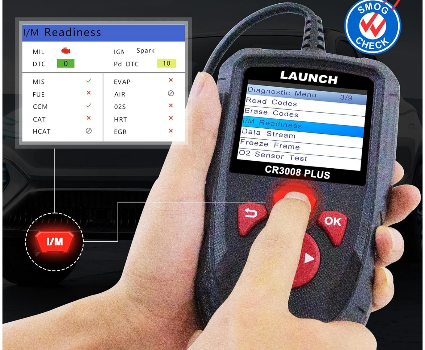
Image: The LAUNCH CR3008 Plus performing a one-click I/M Readiness test, indicating system status for emission checks.
