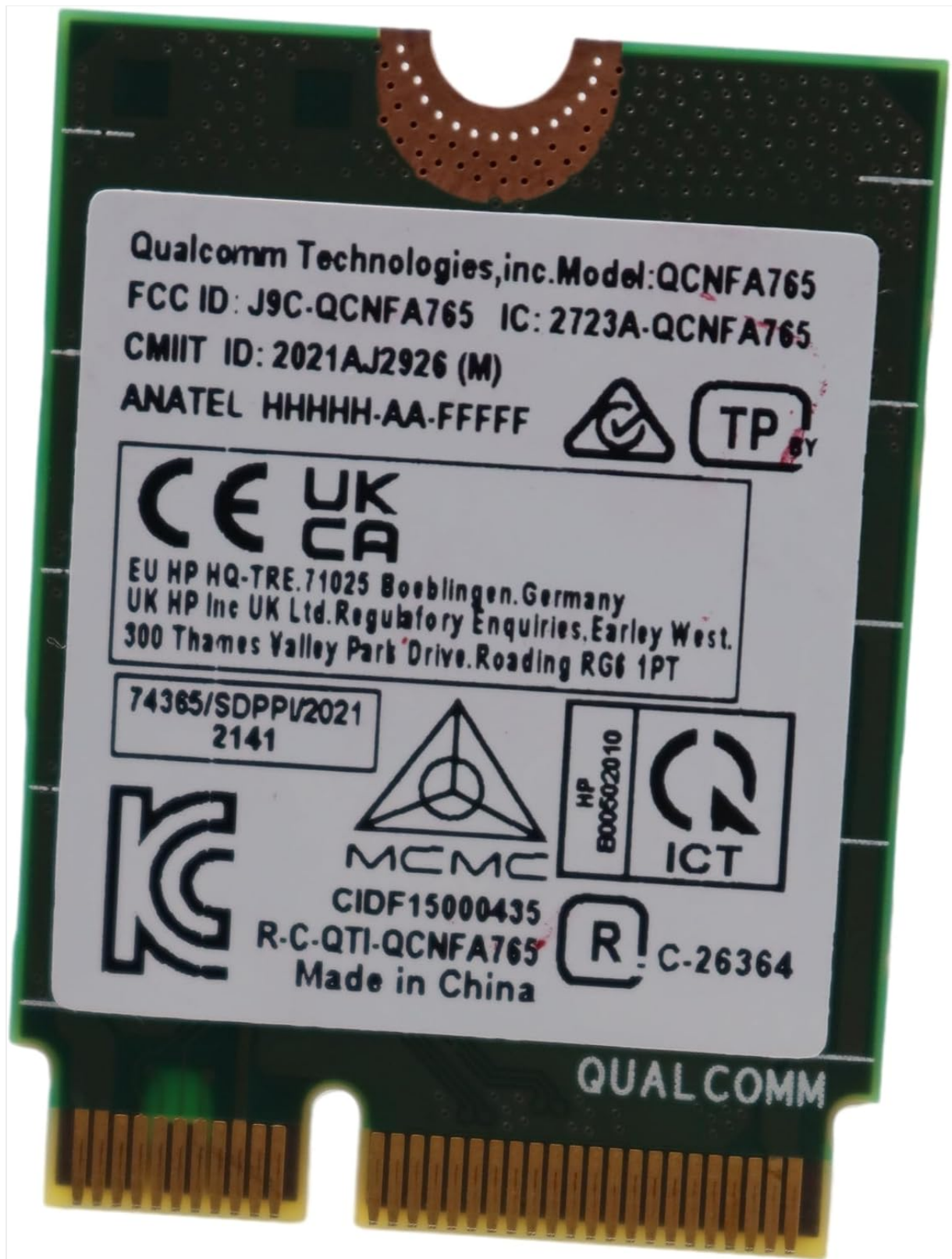
Figure 2: Close-up of the NFA765A card showing connectors
