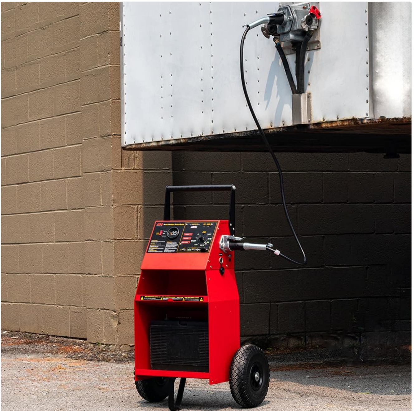
Figure 2: Smart MUTT X connected to a trailer for testing.
