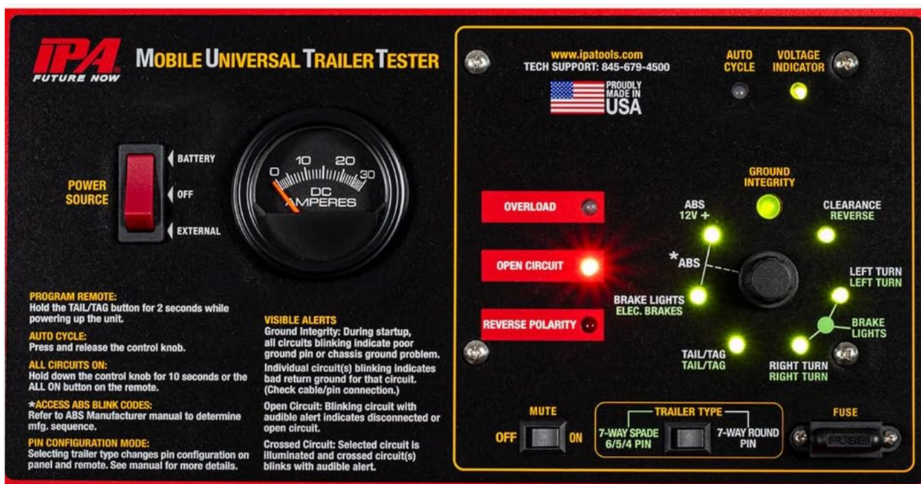
Figure 4: Detailed view of the Smart MUTT X control panel with indicators and controls.
