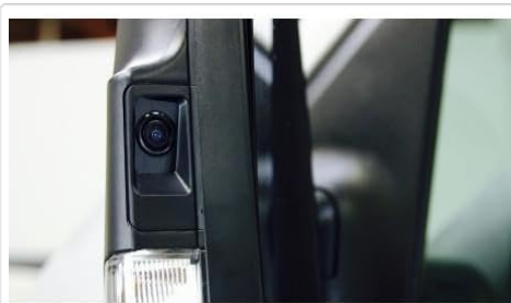
Image 3: The blind spot camera system installed
