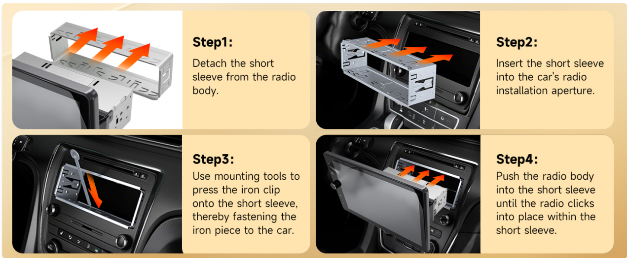
Figure 3.2: Stereo mounting steps.
