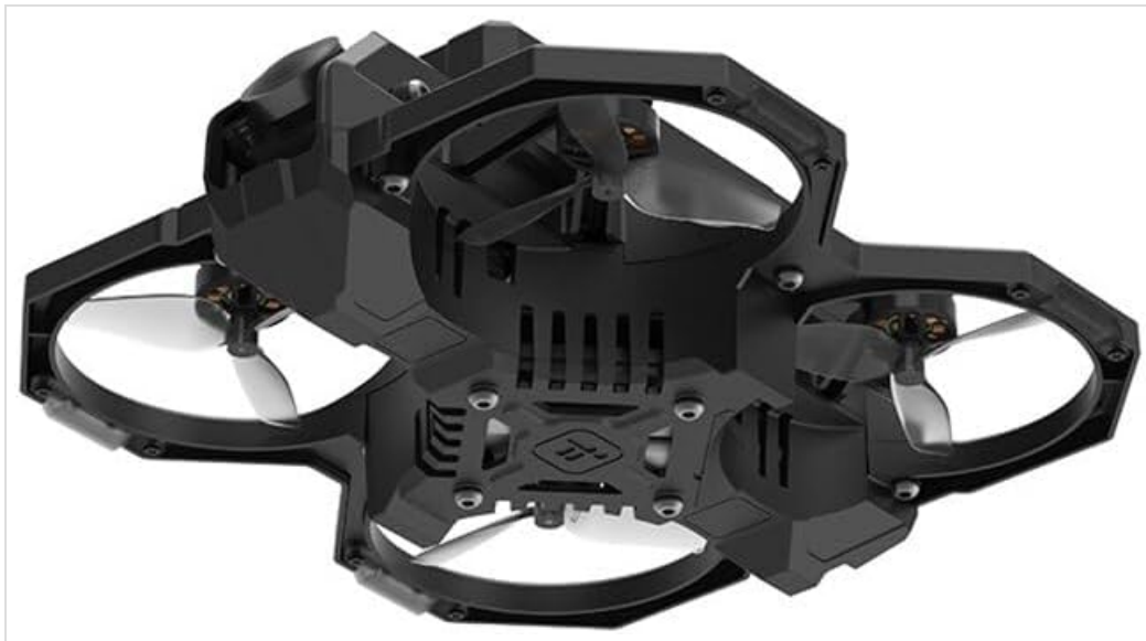
Figure 2: Bottom view of the iFlight Defender-16 drone, highlighting the motor mounts and frame structure.
