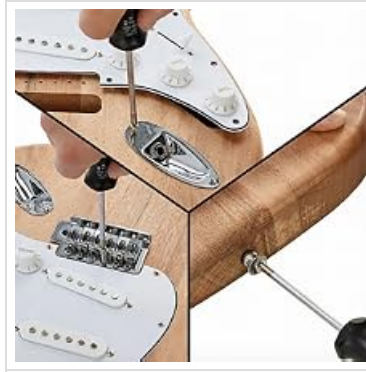
Image: A hand using a screwdriver to secure the guitar bridge to the body.
