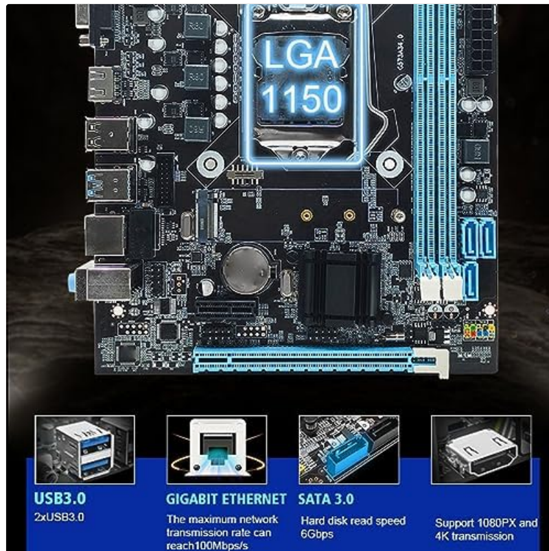
Image: The ASHATA H81 MATX Motherboard with callouts for USB 3.0 ports, Gigabit Ethernet, SATA 3.0, and its support for 1080P and 4K display resolutions.
