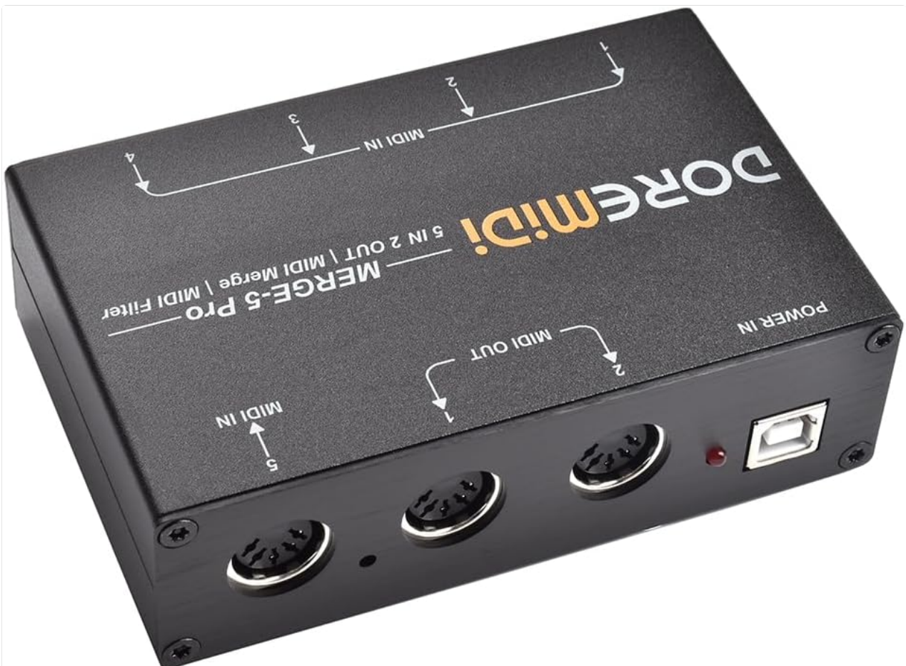
Image: Rear view of the MERGE-5 Pro unit, showing the Power In (USB), MIDI OUT ports 1-2, and MIDI IN port 5.
