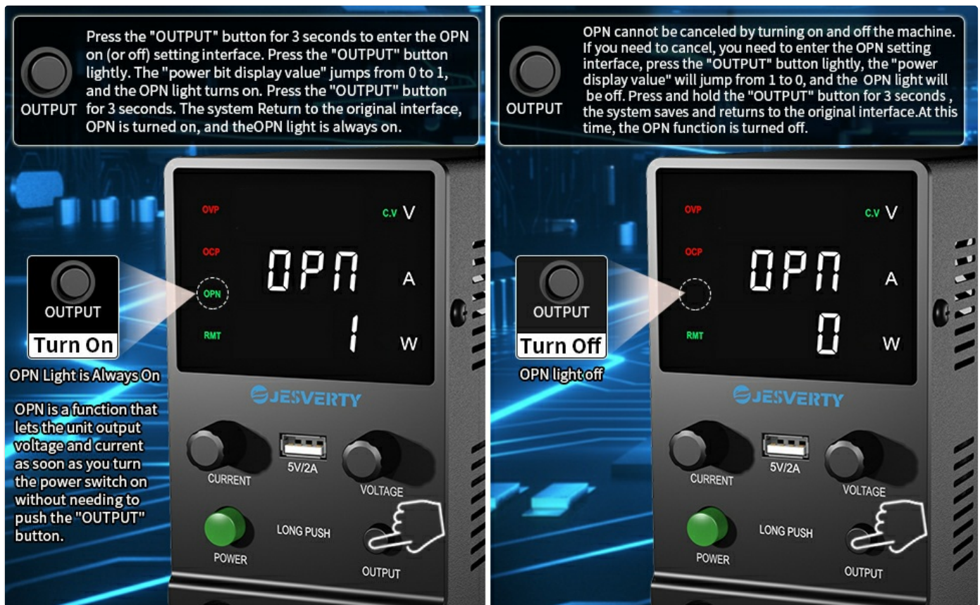
Image: Visual guide for enabling and disabling the OPN (Output Power On) function using the OUTPUT button.
