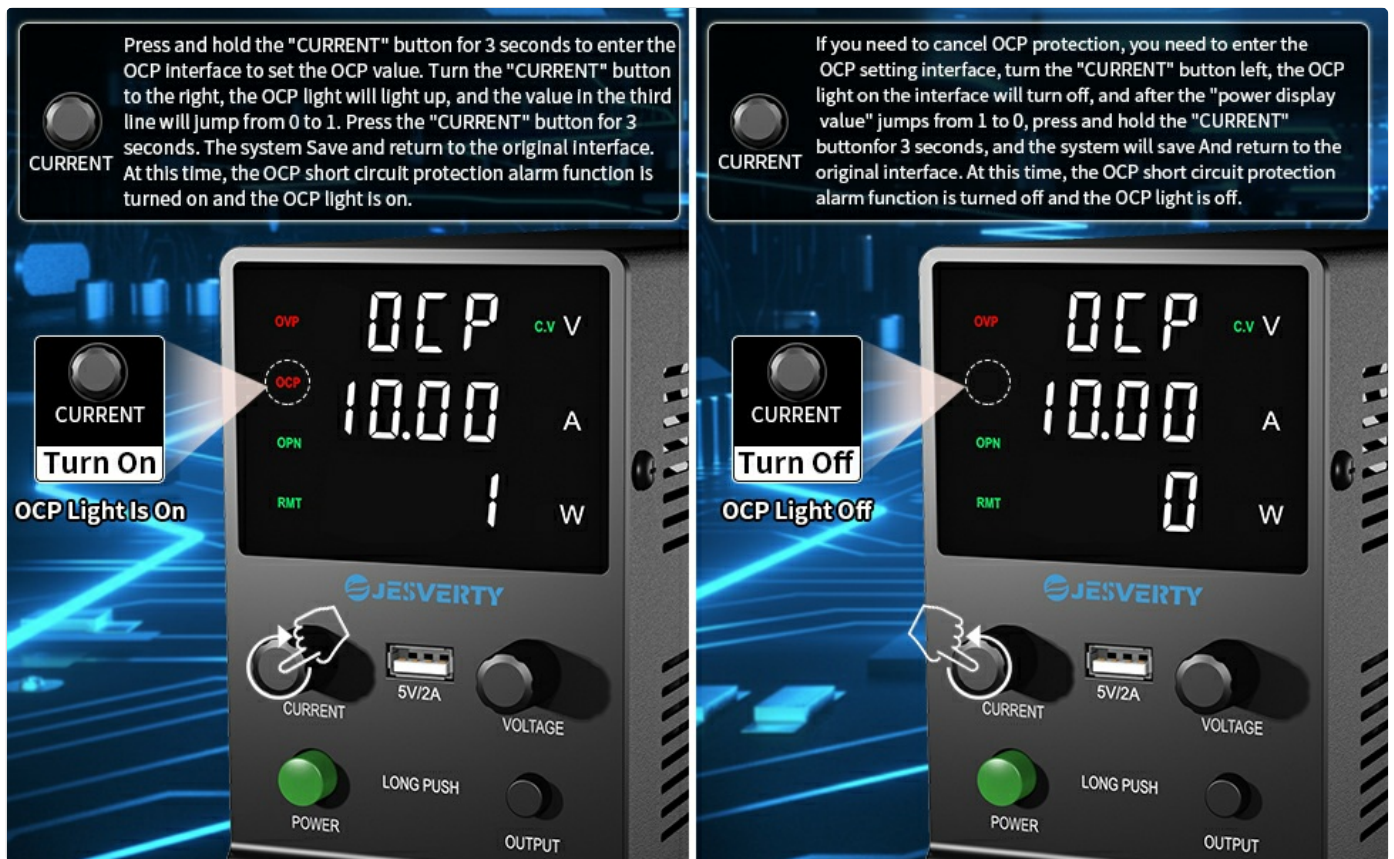
Image: Visual guide for enabling and disabling Over Current Protection (OCP) and setting its value using the CURRENT knob.
