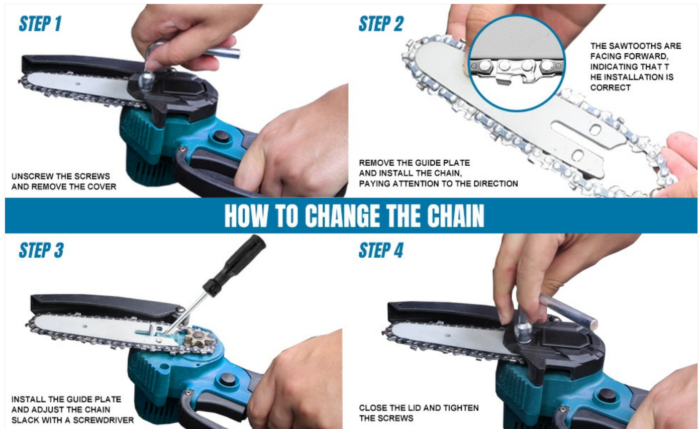
Figure 3.1: How to Change the Chainsaw Chain.
