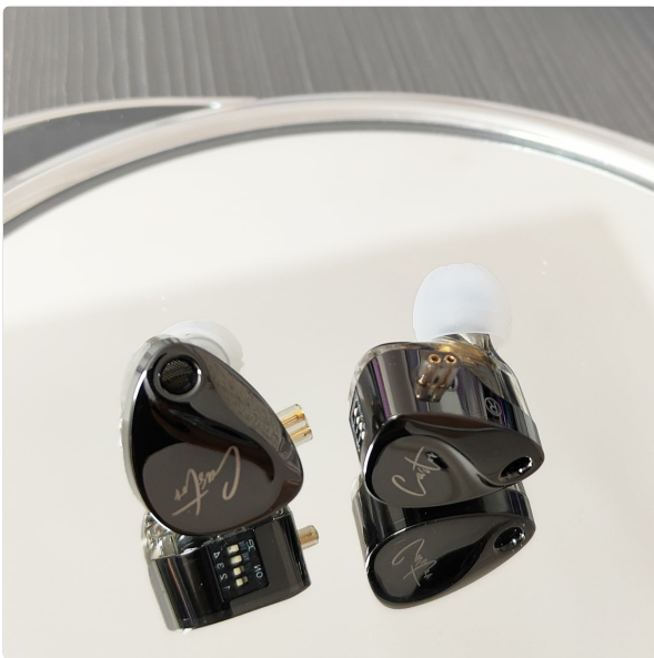
Close-up view of the KZ Castor headphones, highlighting the tuning switches on the side for sound customization.
