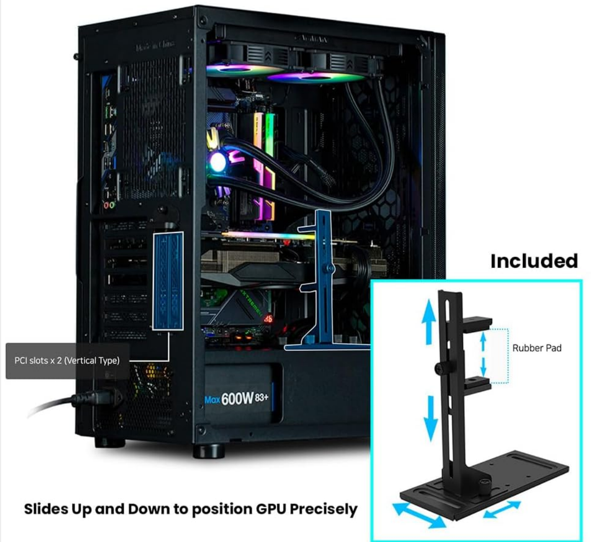
Figure 5: The included height-adjustable GPU support bracket (Zalman VS-1) installed within the case, designed to prevent graphics card sag.
