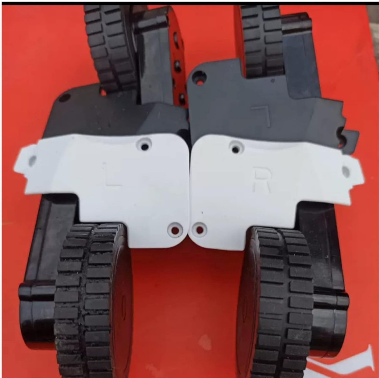
Image 3: Two CONVOW robotic vacuum cleaner wheel assemblies, showing the top housing with 'L' and 'R' markings for Left and Right. These markings assist in correct orientation during installation.
