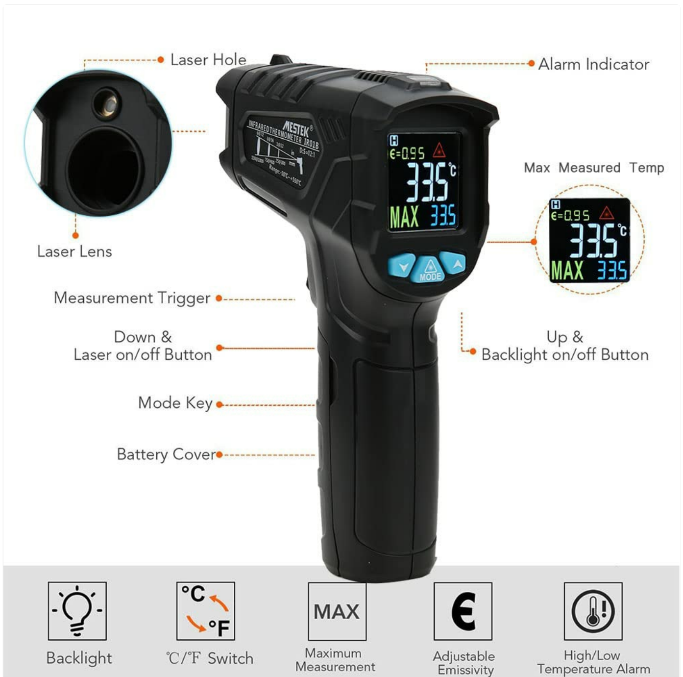
Figure 3: Labeled diagram of the Infrared Thermometer's components.
