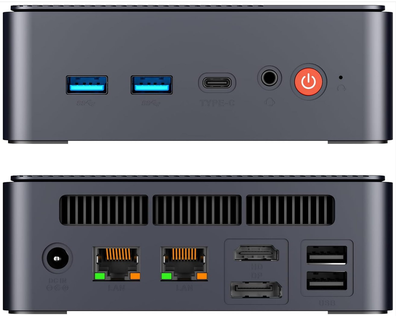
Image 3.1: AWOW Mini PC Front and Rear Ports. This image details the front ports (2x USB 3.2, Type-C, Audio 2-in-1, Power Button, CMOS Reset) and rear ports (DC IN, 2x LAN, HDMI, DP, 2x USB 2.0).
