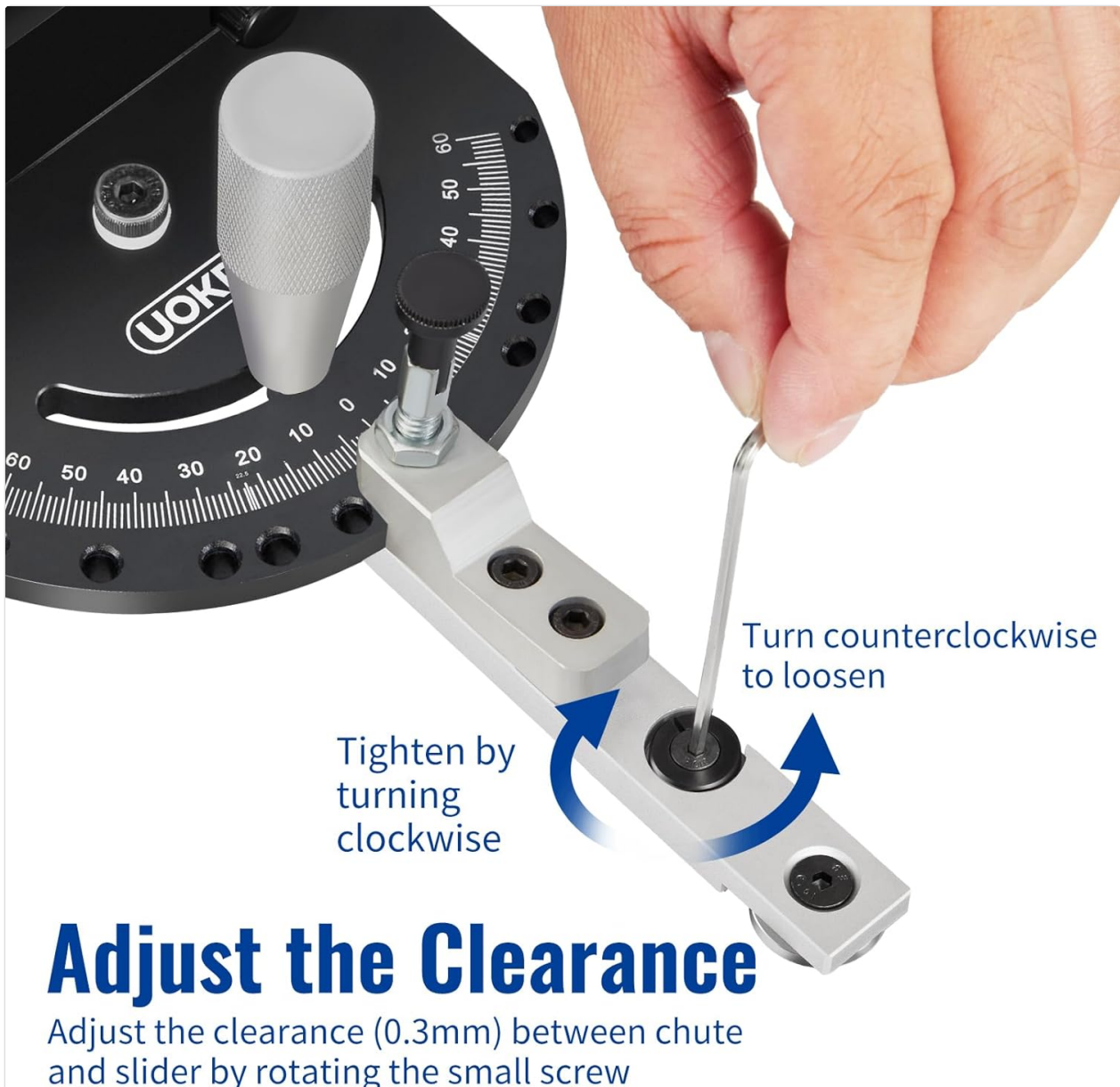
Figure 4: Image demonstrating how to adjust the clearance of the miter bar using an Allen wrench. Turning clockwise tightens, counter-clockwise loosens.
