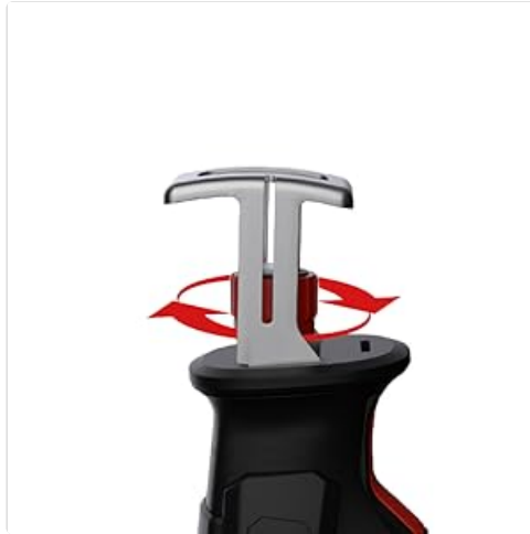
Image 4.2: Turn the locking sleeve counter-clockwise to open the blade holder.
