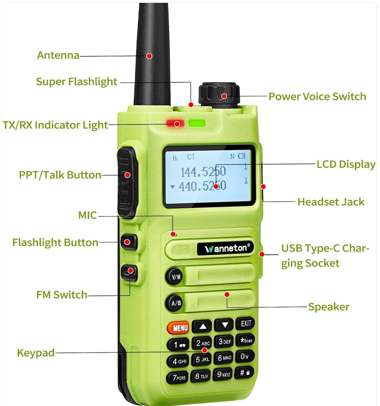
Image: A detailed diagram of the Wanneton UV5F radio, with labels pointing to key components such as the Antenna, Super Flashlight, TX/RX Indicator Light, PTT/Talk Button, MIC, Flashlight Button, FM Switch, Keypad, Speaker, USB Type-C Charging Socket, Headset Jack, LCD Display, and Power Voice Switch.
