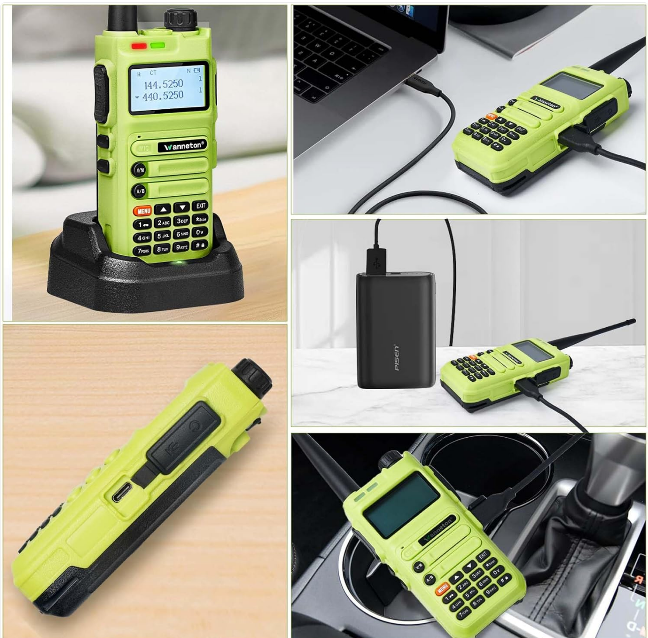
Image: Various charging methods for the Wanneton UV5F radio, including charging in its desktop cradle, via USB-C from a laptop, and via USB-C from a power bank or car charger.
