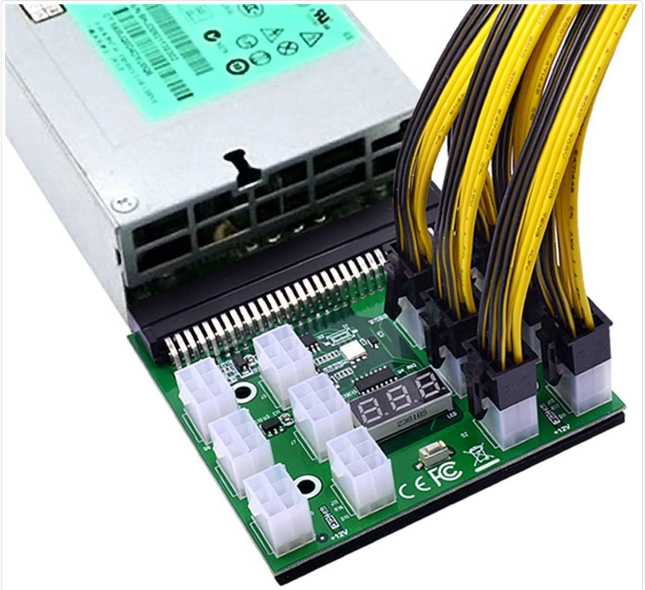
Image: The KLVN Power Module Breakout Board securely connected to a compatible server power supply unit (PSU).
