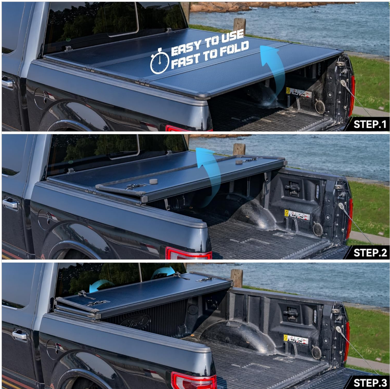
Figure 3: Step-by-step illustration of the cover's folding mechanism.
