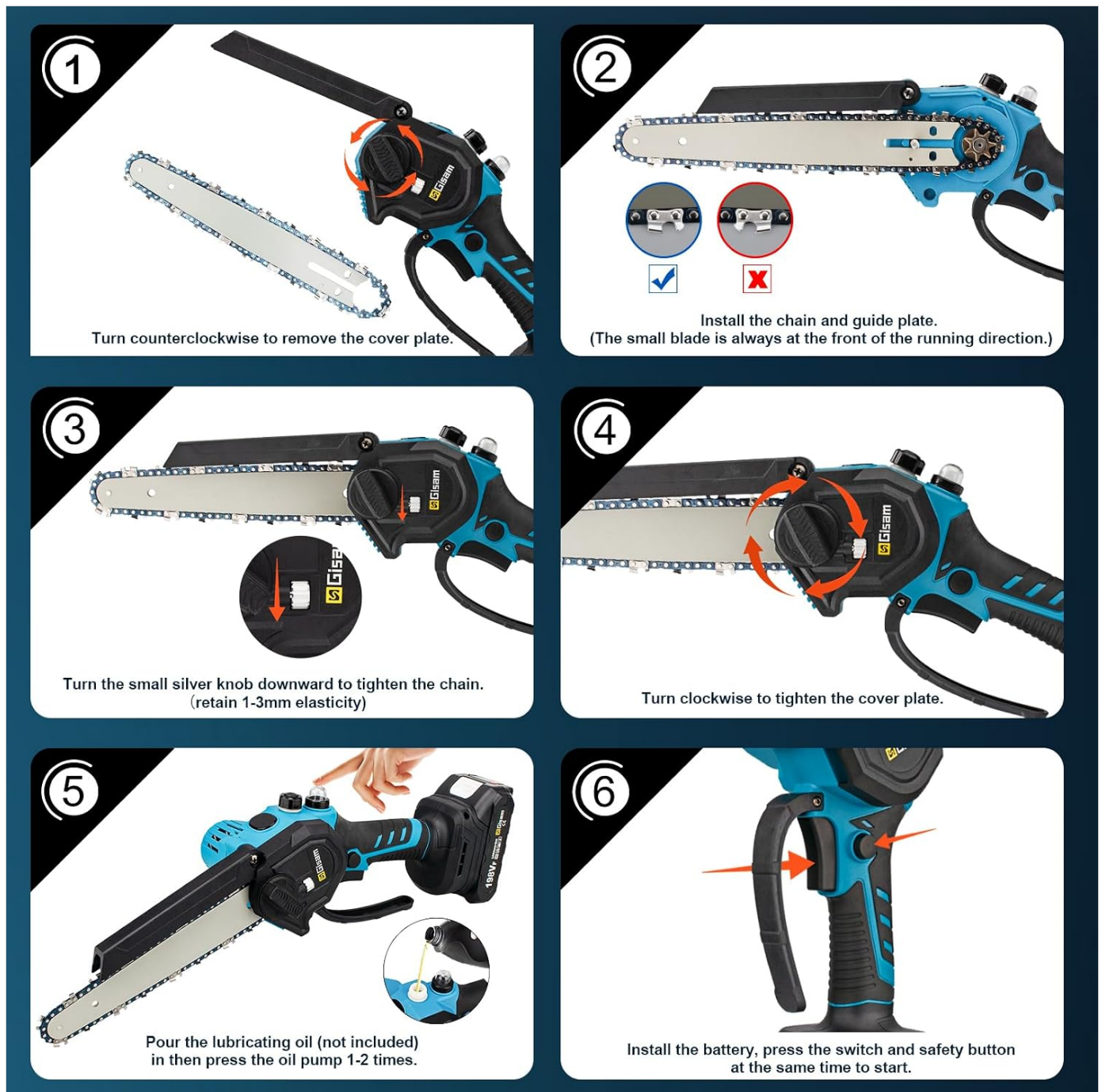
Figure 2: Step-by-step guide for installing the chain and guide plate (1-4), lubricating the chain (5), and starting the chainsaw (6).
