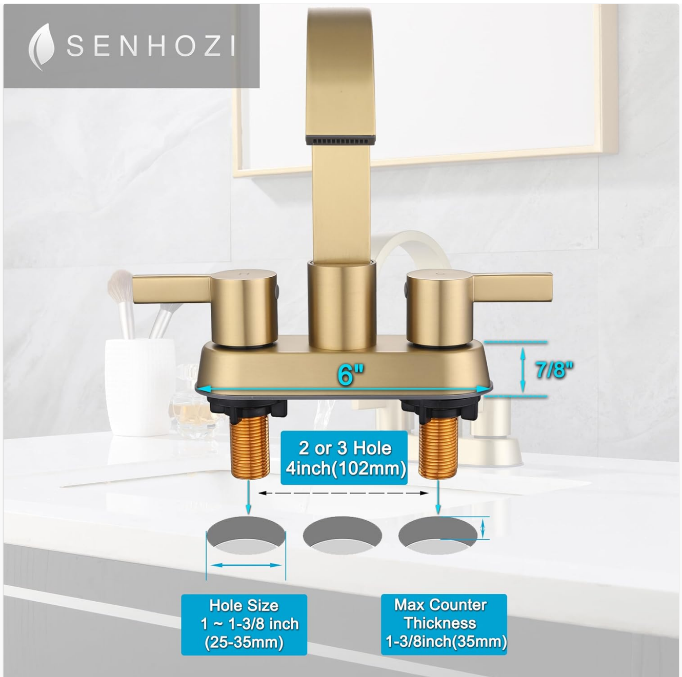
Image 4.2: Sink hole and counter thickness requirements.
