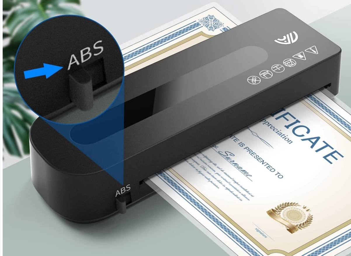
Figure 6.3: Detailed view of the ABS release lever. To use, push the lever to the left and hold it until the jammed paper or pouch can be safely pulled out from the laminator.
