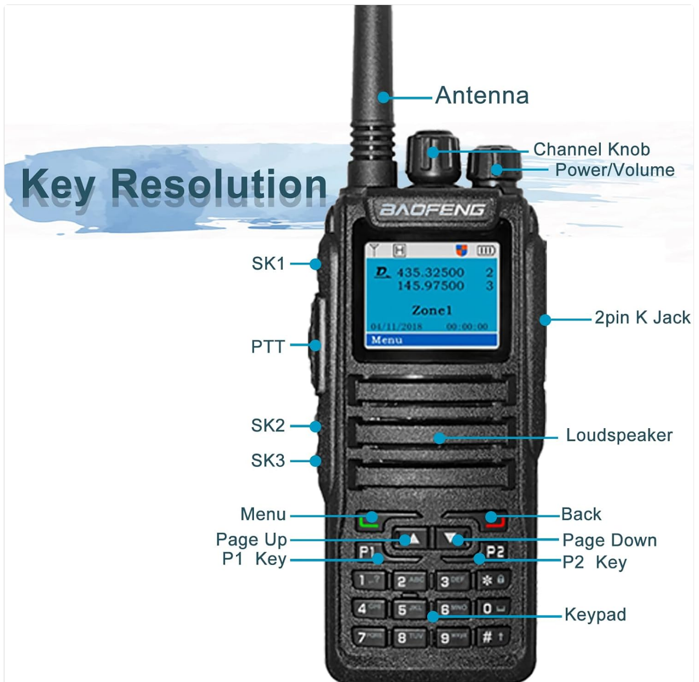
Figure 4.1: Labeled diagram of the BAOFENG DM-1701 radio components.
