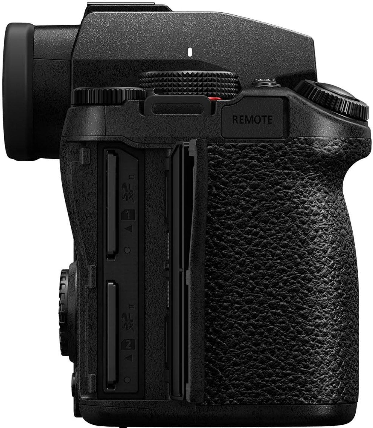
The right side of the camera, revealing the dual SD card slots for extended storage and backup capabilities.
