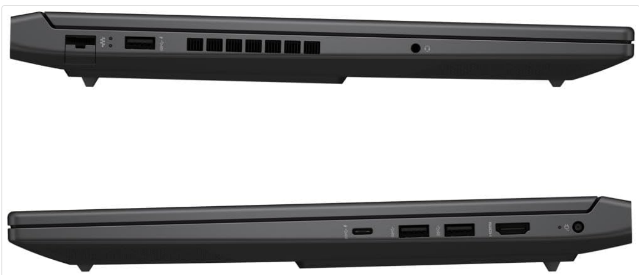
Figure 4.5: Side profiles of the HP Victus 16.1" Gaming Notebook, detailing the placement of various input/output ports and ventilation grilles.
