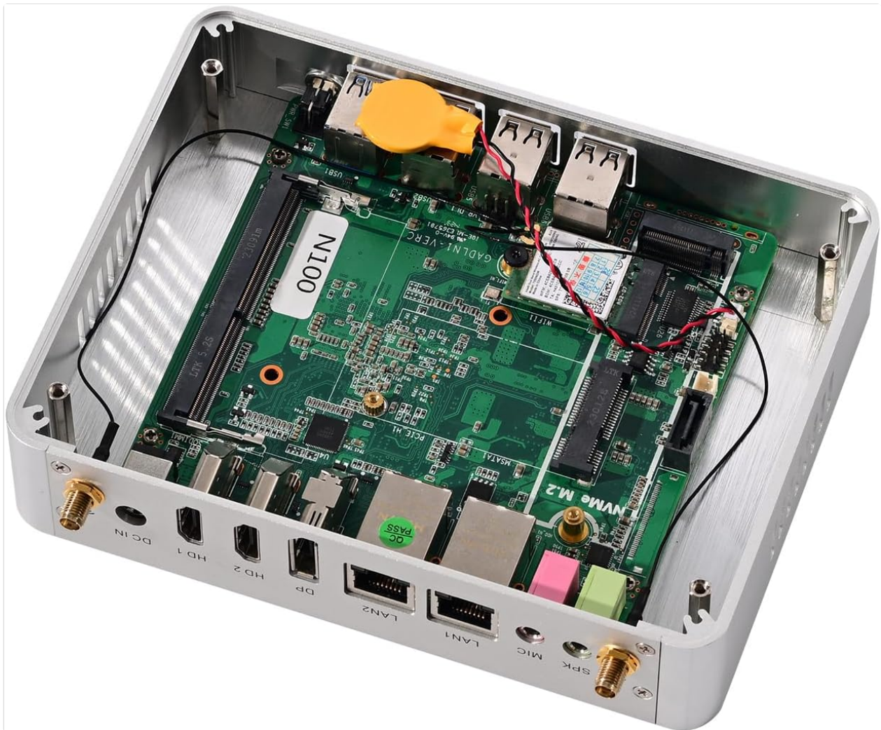
Figure 2.4: Internal view of the HUNSN BM34 Mini PC, showing the motherboard, RAM slot, and storage interfaces.
