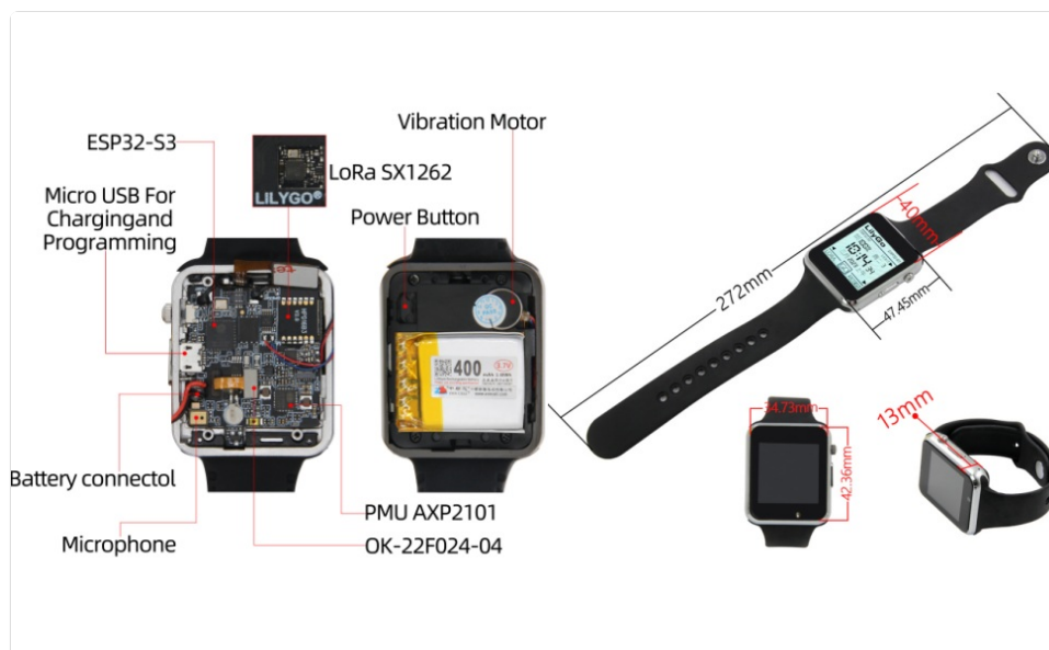
Figure 3.3: Internal and external components of the T-Watch-S3.
