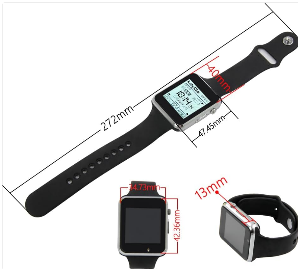
Figure 4.1: Physical dimensions of the T-Watch-S3.
