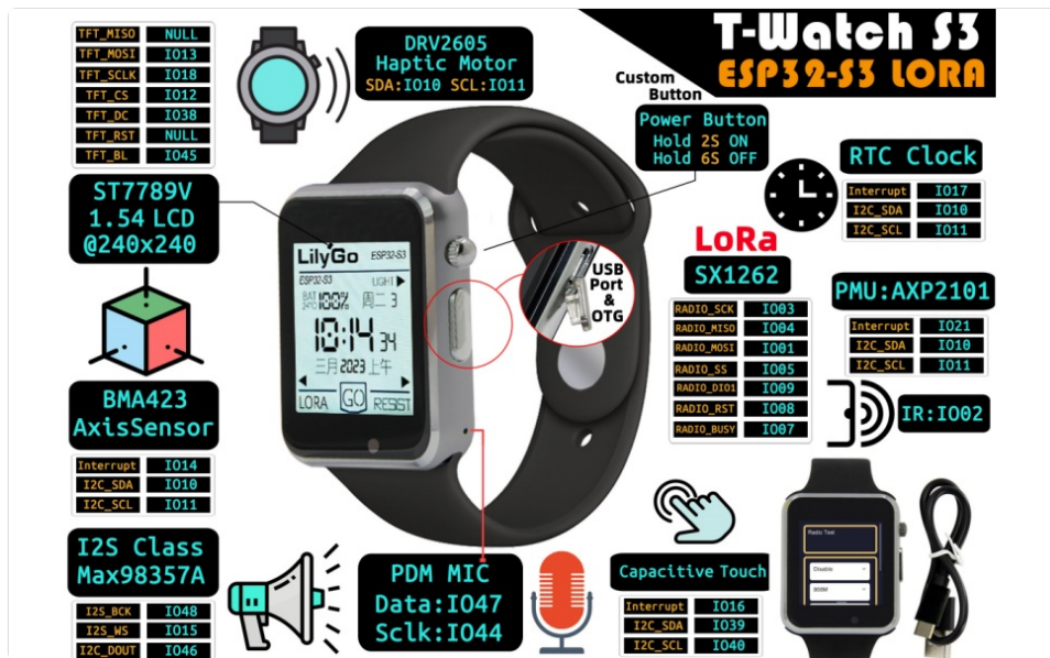
Figure 3.4: Detailed component and pinout diagram.
