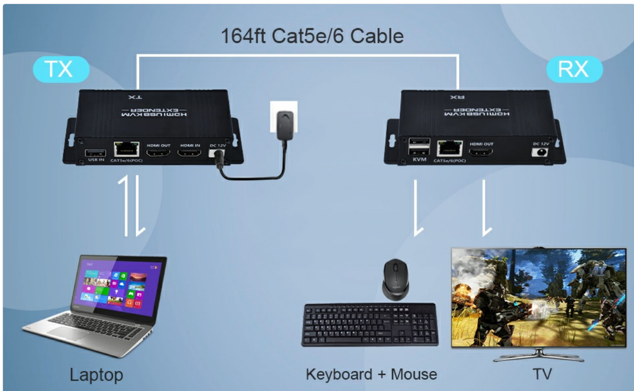
Image 4.1: Connection diagram illustrating how to connect the Transmitter (TX) to the source PC and local display, and the Receiver (RX) to the remote display, keyboard, and mouse via a Cat5e/6/7 cable.
