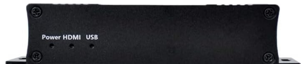
Image 8.1: The dimensions of a single extender unit are 4.56 inches in length, 1.96 inches in width, and 0.95 inches in height.
