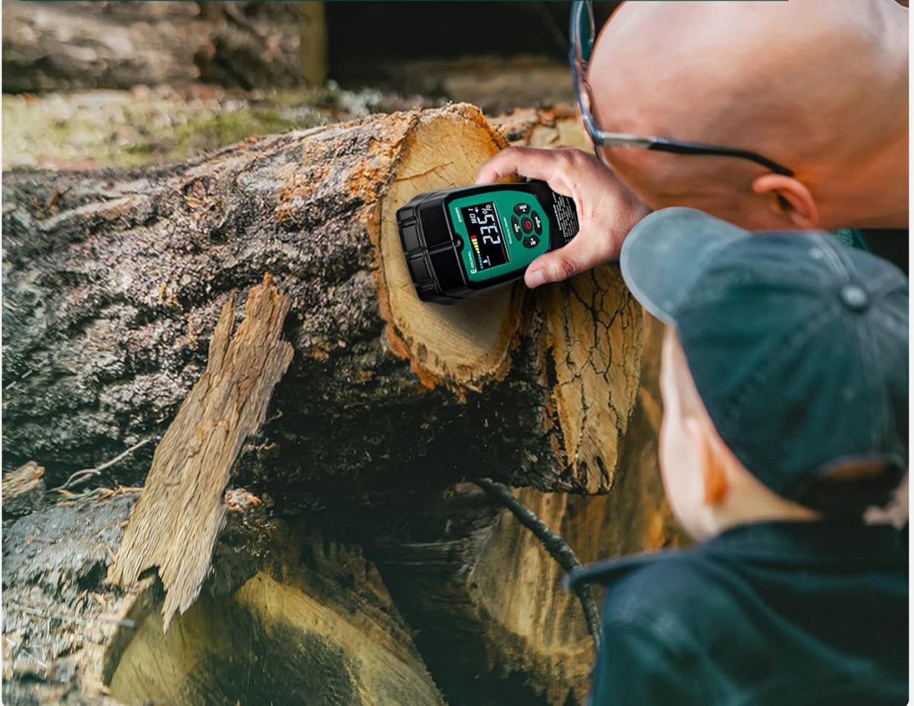
Image: A person using the EWM04 to measure moisture in a large log, demonstrating practical application.
