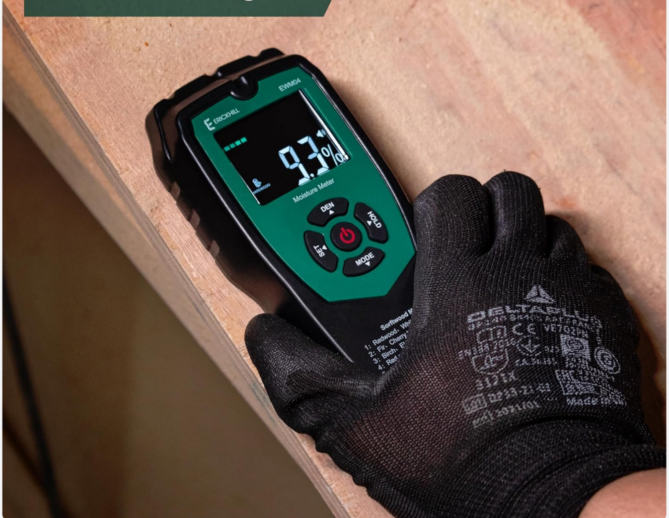
Image: A close-up of a hand holding the meter against a wooden surface, showing the non-destructive measurement process.
