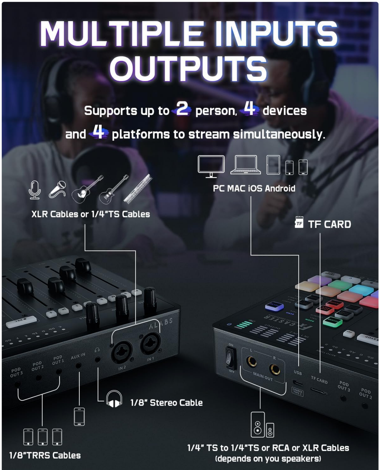
Figure 3: Diagram illustrating the various input and output connections on the Fxcaster, including XLR, 1/4-inch TS, 1/8-inch TRRS, USB-C, and TF card slot, compatible with PC, Mac, iOS, and Android.
