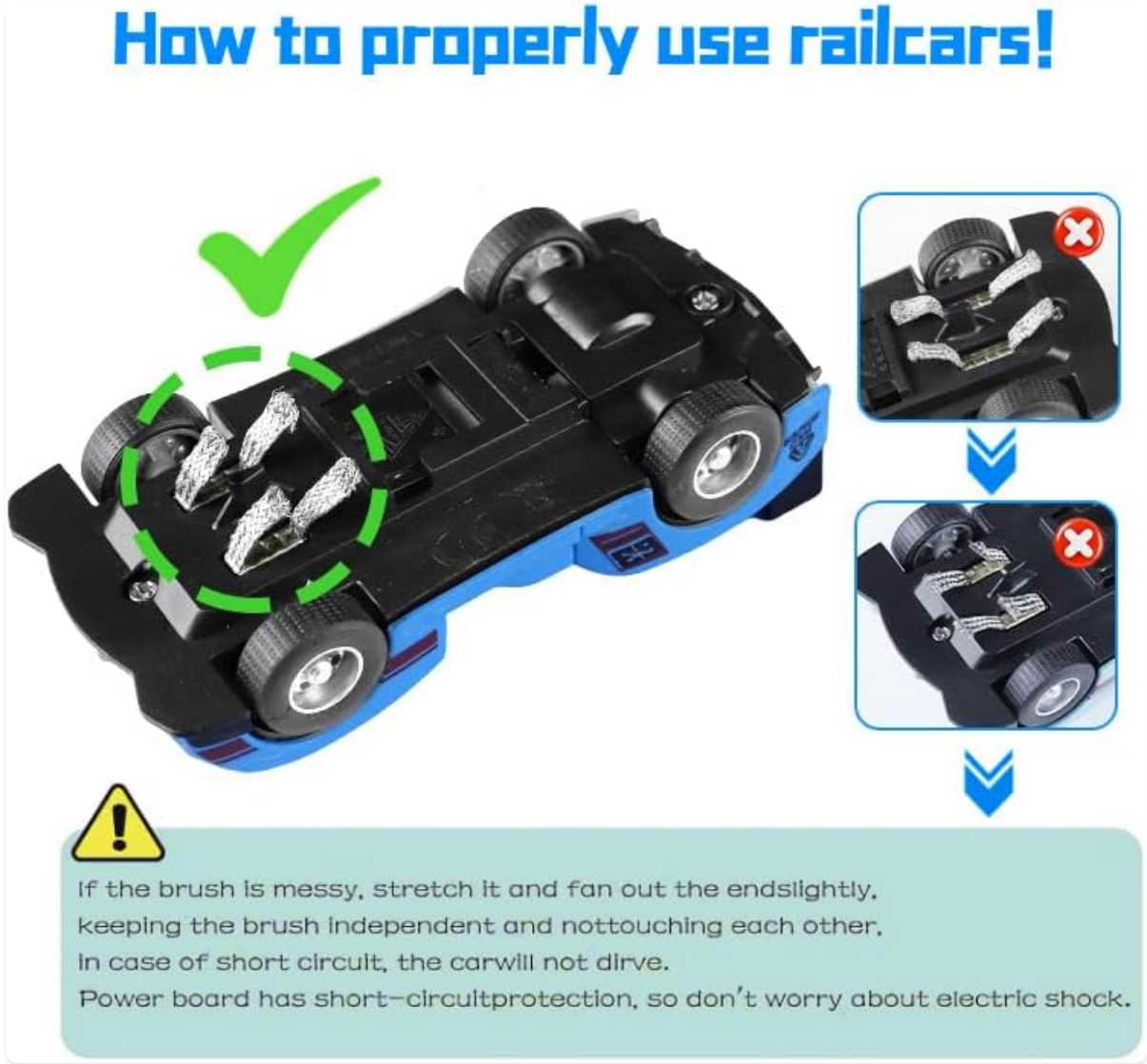
Figure 11: Guide for maintaining slot car brushes.
