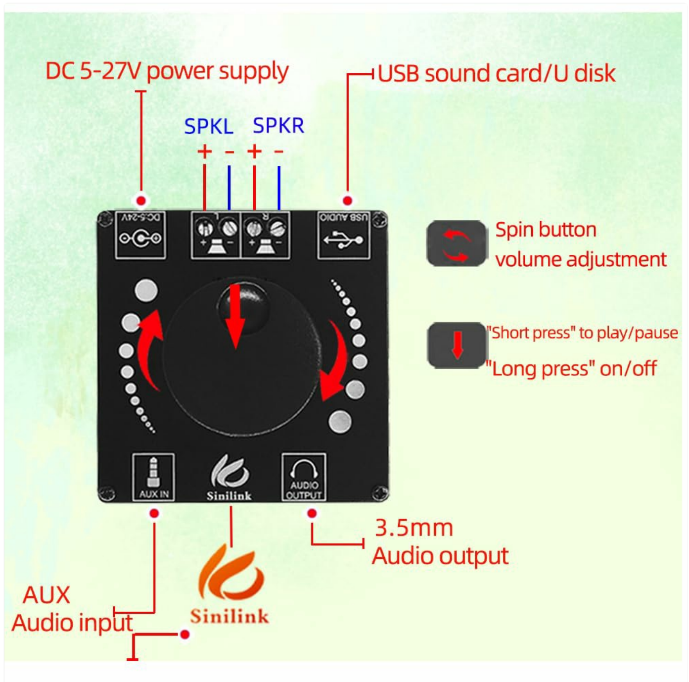
Figure 2: Connection diagram for the XY-AP50H amplifier board. This diagram illustrates the proper connections for DC power, speakers, AUX input, USB audio, and audio output.
