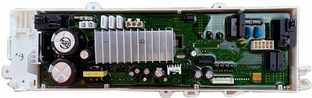
Image 1: NieKe Washing Machine Motherboard Control Board (DC92-01768C). This image shows the general appearance of the control board, highlighting its various connectors and components. It is crucial to match the new board's layout with the old one and ensure all connections are correctly made during installation.
