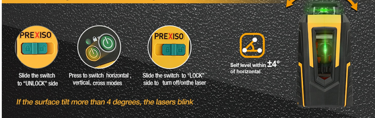
Image: A visual guide demonstrating the steps for activating and using the Self-Leveling Automatic Mode, including the switch position, power button function, and the blinking alarm for out-of-level conditions.
