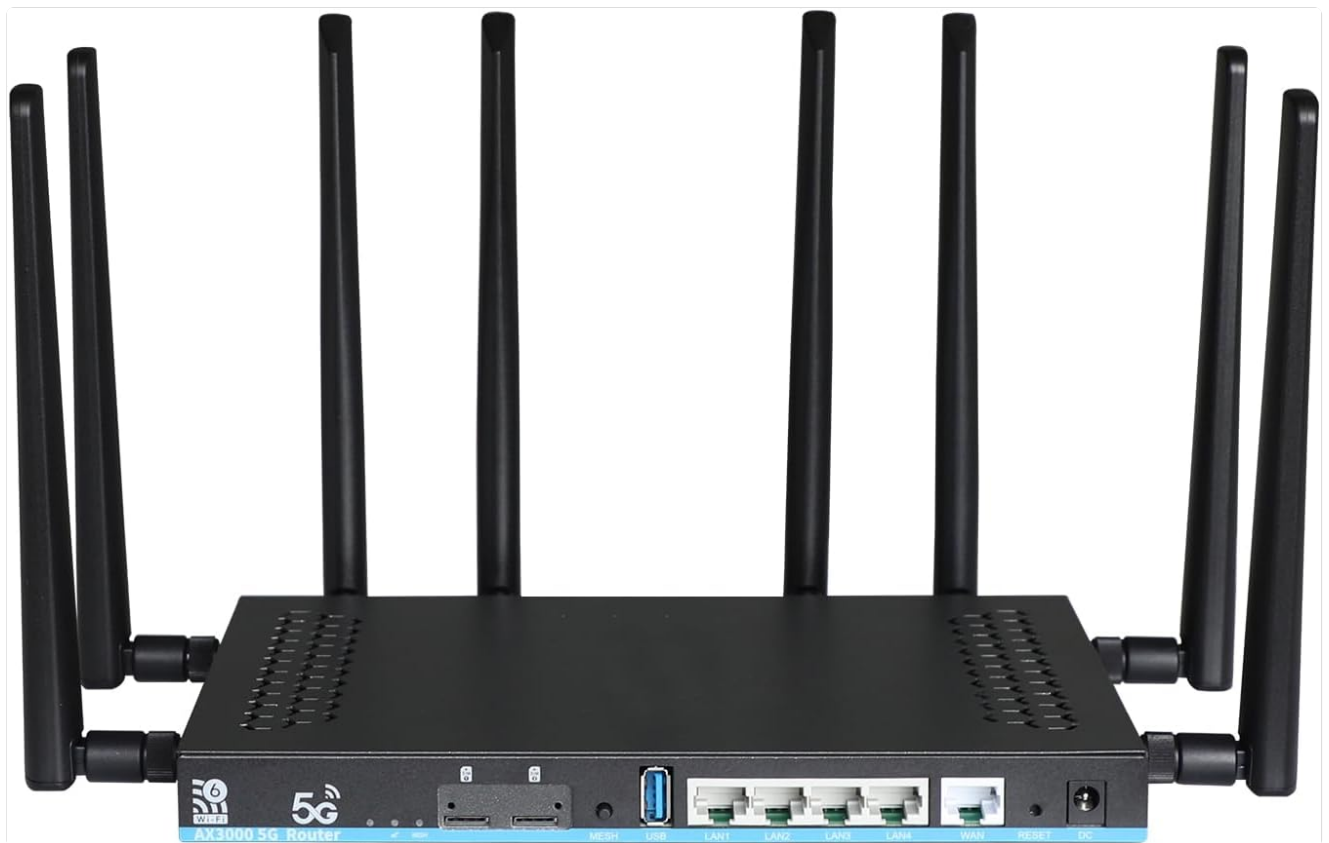
Image: The router with all eight antennas securely screwed into their respective ports.
