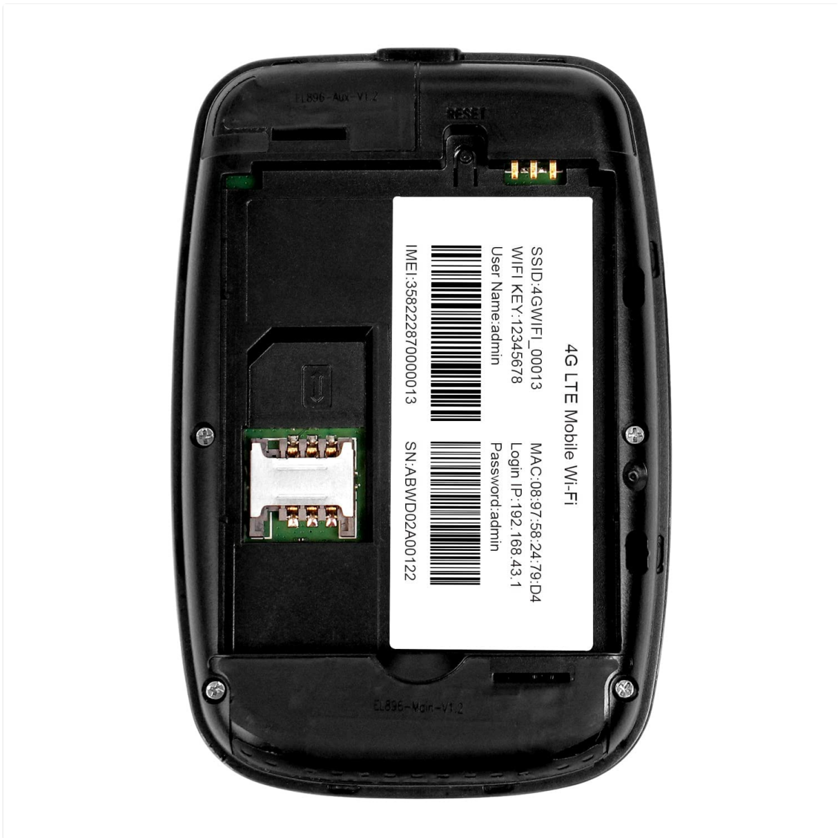
Figure 4: Internal label displaying default Wi-Fi SSID and Key.
