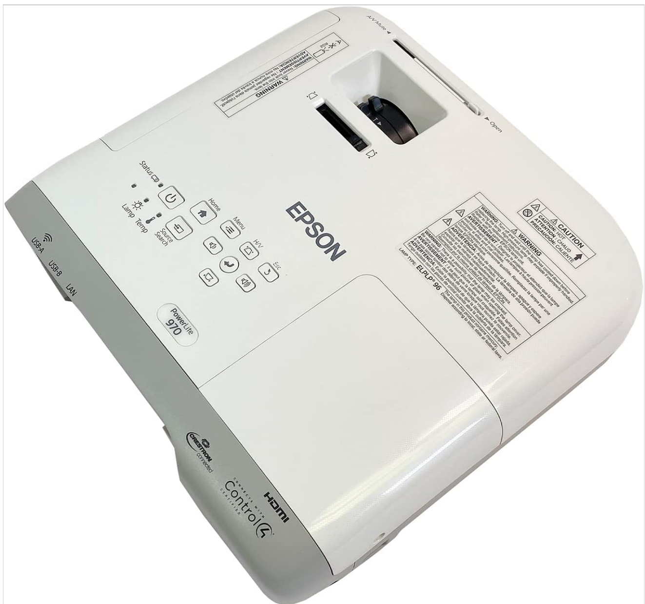
Image: Side view of the Epson PowerLite 970 projector, highlighting the lamp access cover, which can be removed for lamp replacement.
