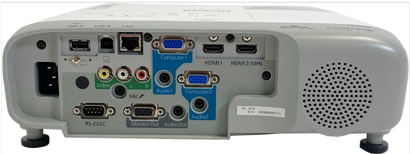
Image: Rear panel of the Epson PowerLite 970 projector, displaying connectivity options including HDMI 1, HDMI 2/MHL, Computer 1 (VGA), Computer 2 (VGA), Video (RCA), Audio 1, Audio 2, Mic, Monitor Out, Audio Out, RS-232C, USB-B, USB-A, and LAN.
