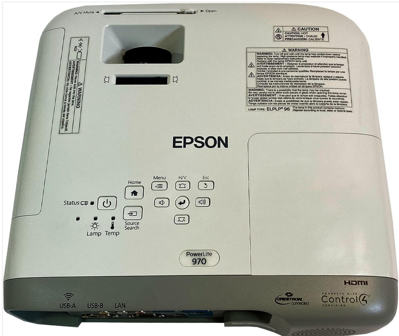
Image: Top panel of the Epson PowerLite 970 projector, showing the control buttons including Power, Menu, Home, Source Search, A/V Mute, and navigation keys, along with focus and zoom rings.
