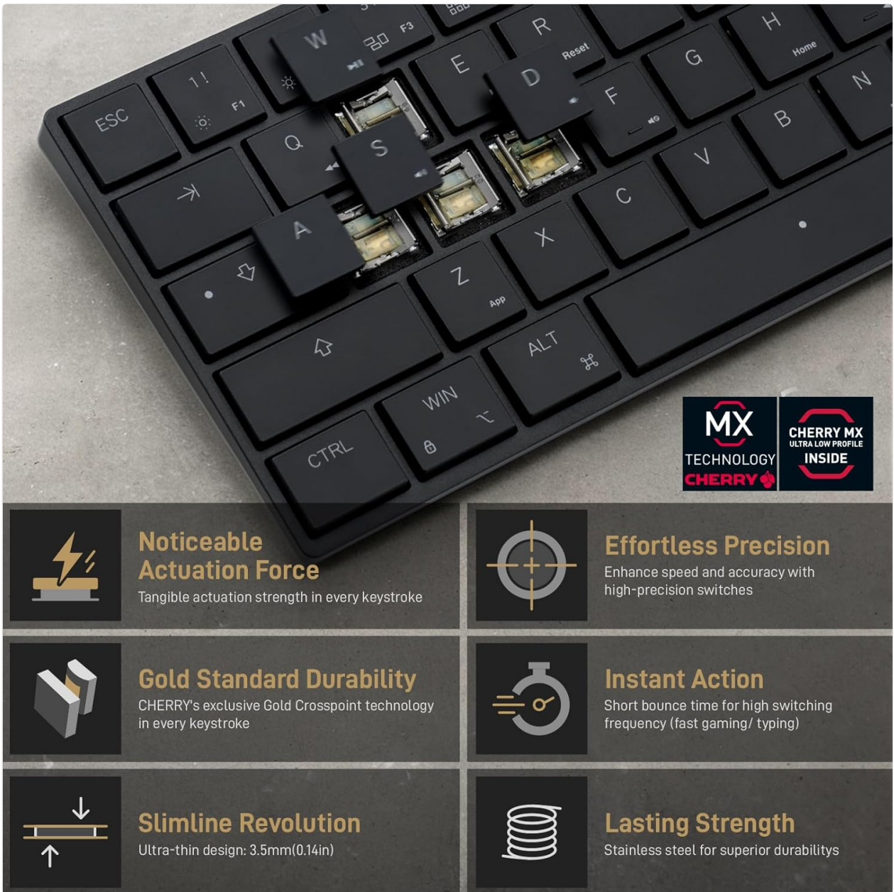
Image 7.1: A detailed view of the Cherry MX Ultra-Low Profile switches, highlighting their precision engineering.
